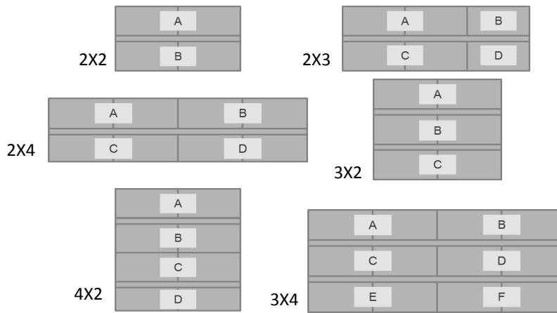
All bin configurations are set up with zones, which correspond to a set of heaters that work together to hold the product. A single product can be programmed into each zone.
