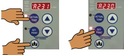
**4** Press the **UP** or **DOWN** Arrow button until the temperature displayed matches the reading obtained in Step 2. Press the **CROWN BUTTON** to save the temperature value and exit the Calibration Mode.
