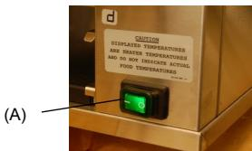
Allow 20 minutes for heaters to reach operating temperature.
