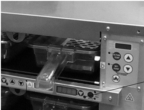
If more than one pan is active for a product, the **LED** for the first pan loaded will turn from **BLANK** to **GREEN**.
