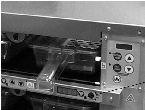
If more than one pan is active for a product, the **LED** for the first pan loaded will turn from **BLANK** to **GREEN**.
