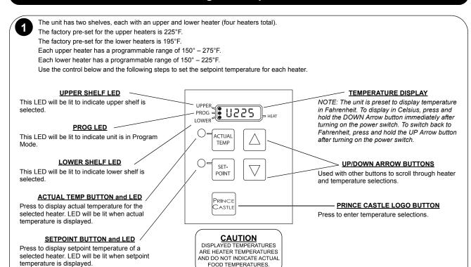
NOTE: To reset all times and temperatures to the factory settings, turn the unit off, then press and hold the UP and DOWN Arrow buttons simultaneously while turning the unit back on. A "P" will appear in the display and all times and temperatures will be reset to original factory settings.
