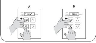
To check the timer address, press and hold the PRINCE CASTLE LOGO button and the DOWN Arrow button. The current timer address will be displayed in the far right timer display. To change the timer address, proceed to Step 6.
