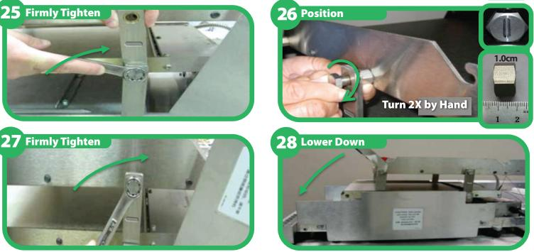
Check accuracy of work by lowering and raising the platens three times. Platens should raise and lower without excessive side to side movements and resistance. Platen bolts should remain in place.
